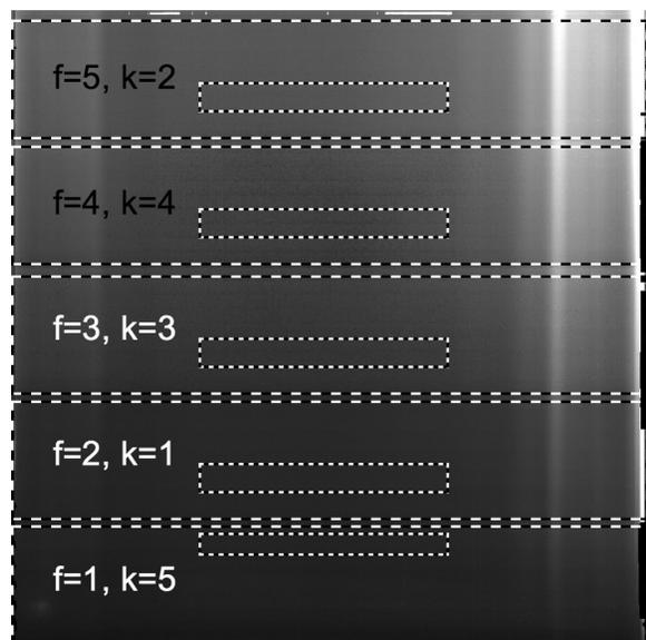
**Figure 9.** Preflight test mode image showing the register signal from the integrating sphere calibration source (using nine 8 W lamps), with each filter labeled with its filter ( $f$ ) and band ( $k$ ) number. The large boxes outline the regions of the detector from which the  $1024 \times 192$  framelets for each filter are extracted. The smaller boxes show the boundaries of the C-ROI for each filter.
